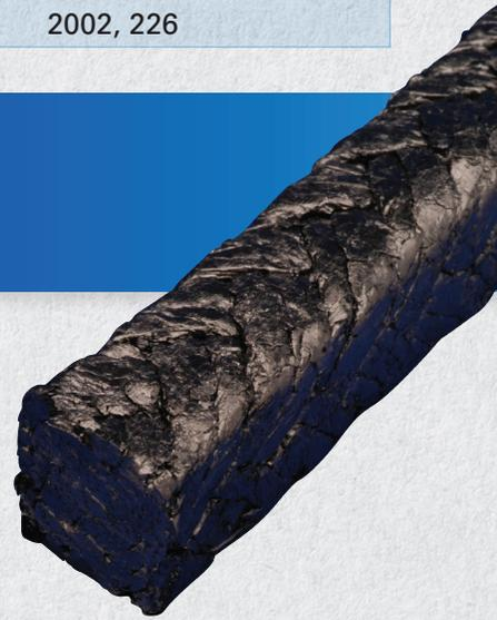
Braided from high purity graphite yarns, Style 5000 is designed to be virtually leak free. Under gland pressure, Style 5000 forms a homogenous mass, resulting in maximum sealability, and reducing flush water usage. Style 5000 packing is also a low friction, self-lubricating packing, with extremely low friction, and excellent heat dissipation. Typically used for high temperature pump or valve applications.
