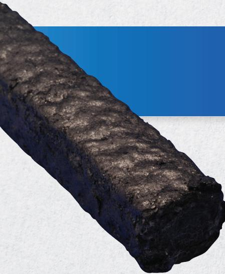
Braided from continuous Acrylic blended fiber, Style 3000G is impregnated with our proprietary high temperature lubricant, and pre and post lubricated with high purity graphite flake. Our unique lubrication process insures a dense but flexible general service packing, which can be used in most steam, water, salt water, oil, and mild acid or alkali applications.
