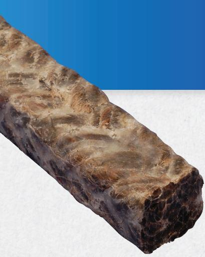
Style 921 is braided from a long lasting blend of Flax and Ramie fibers, than thoroughly lubricated with a proprietary Tallow and Wax blend. A low friction, economical, general service packing used extensively on shipboard applications for stern tubes, rudderposts, and water pumps. This packing is especially resistant to cold water, seawater, and cold oils, but is also used in a variety of other applications in the pulp and paper, marine, and wastewater industries.
