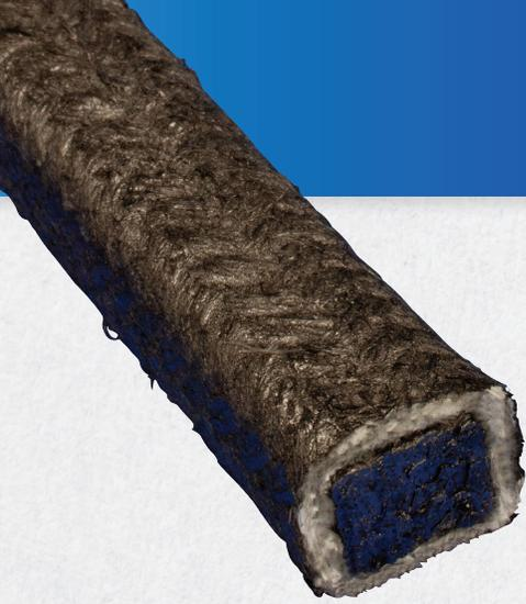
Braided from Inconel® wire inserted fiberglass over a proprietary core, and surface coated with our graphite blend, Style 3030INA is an economical substitute for more expensive steam packing. Style 3030INA packing also contains a corrosion inhibitor to internally protect the valve from oxidation. For use as a high temperature and pressure valve stem or expansion joint packing.
