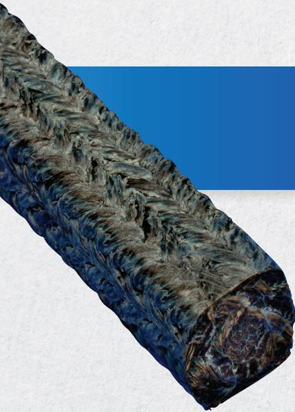
Braided from a blend of carbon yarns, Style 4000 is impregnated with a proprietary blocking agent. Designed to be highly durable and easy to install, Style 4000 packing is also a non-staining, self-lubricating packing. Our unique blend of Carbon yarns ensures extremely low shaft wear, while maintaining excellent heat dissipation. Typically used for severely caustic or corrosive media, this packing is suited for almost any high speed/high temperature pump or valve.
