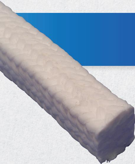
Braided from 100% PTFE filament, Style 344BIL is thoroughly impregnated with a PTFE suspensoidal blocking agent and our proprietary break in lube. Our unique blend of lubricating oil eases friction during startup and operation. A soft but dense and stable packing, 344BIL is ideally suited for chemical process pumps where extreme chemical resistance and extremely low shaft friction are required.
