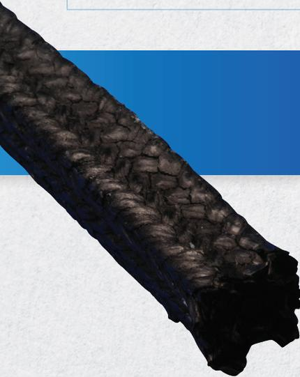
Braided from industrial grade graphite filament, 8000LC is an economical substitute for most braided carbon packing. Coated with our proprietary graphite blend, 8000LC has a low coefficient of friction, as well as extremely high thermal conductivity. For use in valves, centrifugal pumps, rotary pumps, and reciprocating pumps, where the media is highly aggressive or where a high speed shaft packing is needed.
