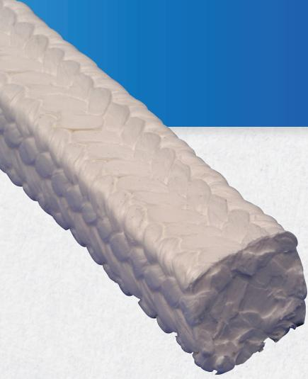
Braided from 100% PTFE filament, Style 344 is then thoroughly impregnated with a PTFE suspensoidal blocking agent. With no sacrificial lubricants to wear out, Style 344 is long lasting, with an extremely low coefficient of friction and excellent heat dispersion. Ideally suited for chemical process applications where extreme chemical resistance is required
